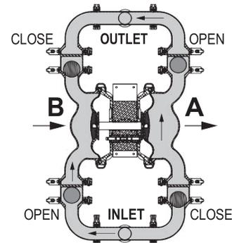
**FIGURE 3** At completion of the stroke, the air valve again redirects air to the back side of diaphragm A, which starts diaphragm B on its exhaust stroke. As the pump reaches its original starting point, each diaphragm has gone through one exhaust and one discharge stroke. This constitutes one complete pumping cycle. The pump may take several cycles to completely prime depending on the conditions of the application.
